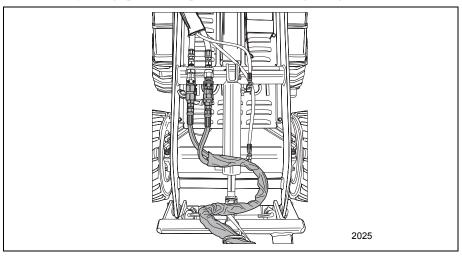
Figure 3-31 Attachment Hydraulic Hose Routing
